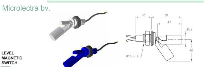
www.microlectra.nl Operating principle The IMN magnetic sensors are based level in the action of a reed switch located inside the tube, which are eneral activated by a magnet housed inside the float and moves due to the thrust of the liquid.
